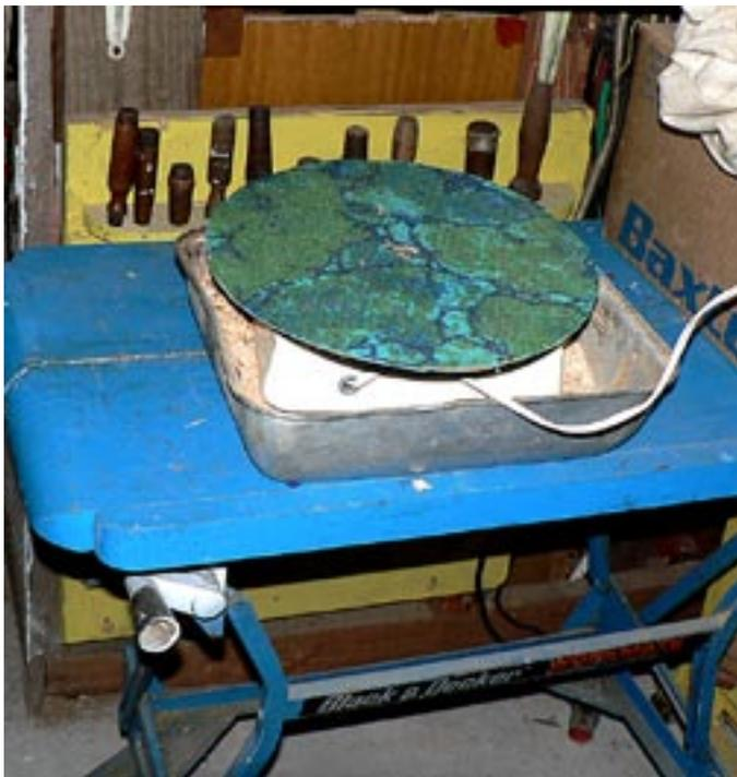
This is a sort of turntable for when you want to work all the way around something. It'll turn 180 degrees one way, then it hits a sort of stop and comes back 180 degrees the other way. I made it out of an old room heater that turns and a piece of carpet.
