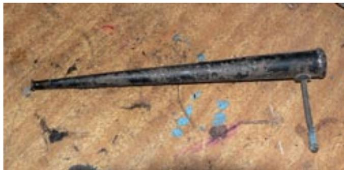
A blowpipe. It was used in the chemistry lab. You'd have your Bunsen burner going, and if you wanted to heat up a crystal or something to break it you put the small end of the pipe near the flame and you blew into the other end, and that directed the flame onto the piece that you wanted heat up.
