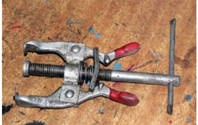
This is a puller specially for removing the battery clips from battery terminals. Sometimes the clips are buggers to get off the terminals, and with this you can pull them off without damaging the terminal.
