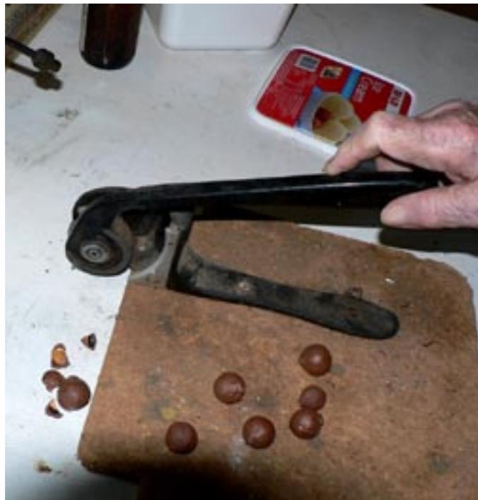
Bet you can't work out what this is for. It's for cracking macadamia nuts. This rounded piece is like a cam that get tighter and tighter as you move the handle, till eventually the nut cracks. I didn't make it, though.
