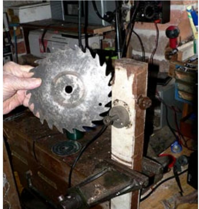
I made this gadget myself. It has provision for sharpening two circular saws. The spindle on the top takes a seven inch saw blade, and the one on the bottom is for a nine and a quarter inch saw blade.
