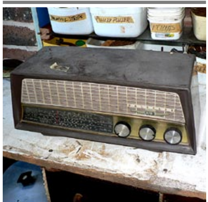
This is a five valve 1960 Kreisher radio. It worked on valves and is powered by an AC cord.
