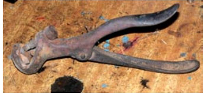
A saw-set. I've got three or four of those. You put it over the tooth of the saw and held it horizontal and when you squeezed it a little piece of metal bent the tooth over to set it so that it wouldn't bind in the cut. It pushed the tooth away from you, so you did every second tooth on one side, then turned the saw around to set every second tooth on the other.
