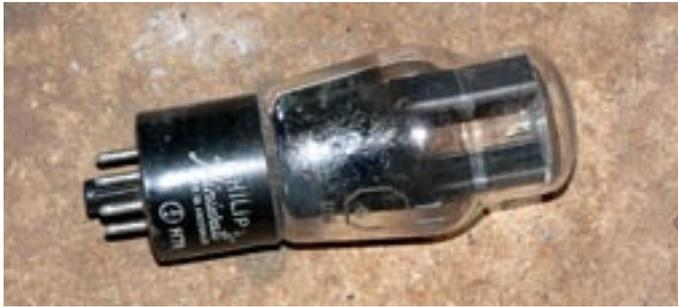
Here we have an Octel valve – that is, a valve with eight pins on the socket at the bottom and a central rod with a keyway on it which would only allow the valve to be inserted in a certain direction. This valve is surrounded by a metal shield which was not only for when the valve was working well, but it was also emitting radio frequency waves which could be picked up by other valves nearby. This meant that it had to be shielded by a metal shield that went around the valve.
