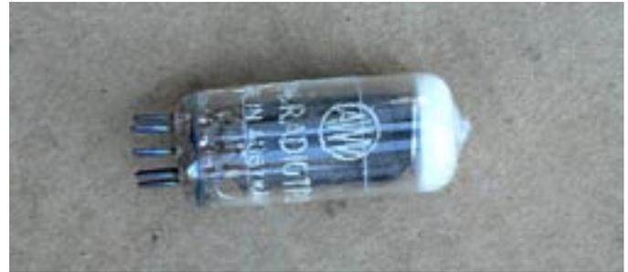
This is a little valve that came out during the war and was used for about twenty years or so. I just included this one because it shows an area of white at the top, which means that air has got into the valve and it is no longer a vacuum – and a vacuum is essential for the working of all valves
