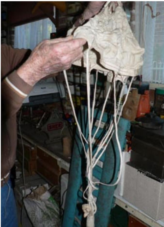
Here is a parachute off the ejector seat of a Sabre aircraft. When you ejected, the seat shot out with the pilot sitting in it. Then he released the seat, and so the seat didn't fall on top of anybody, the parachute let it down gently.
