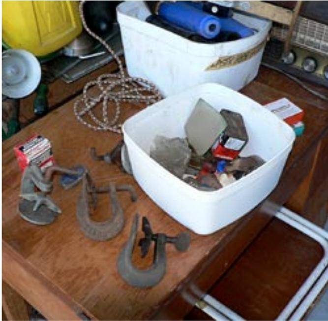
These are vulcanising patches. You used to use them to patch car inner tubes. When you got a puncture you'd scour the spot around the puncture, clamp a special rubber patch over it with these special clamps, then light it, and it would smoulder and fizz away and vulcanise the patch on to the inner tube.
